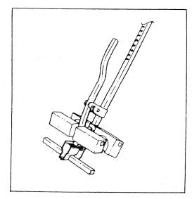
3. Secure LOCKING HANDLE by inserting flat end through ROLL PINS in BOTTOM BRACKET ASSEMBLY. Adjust the HANDLE to the most secure and comfortable position. Push down on HANDLE and bring up to secure ROLL PIN into LOCKING CLIP.
